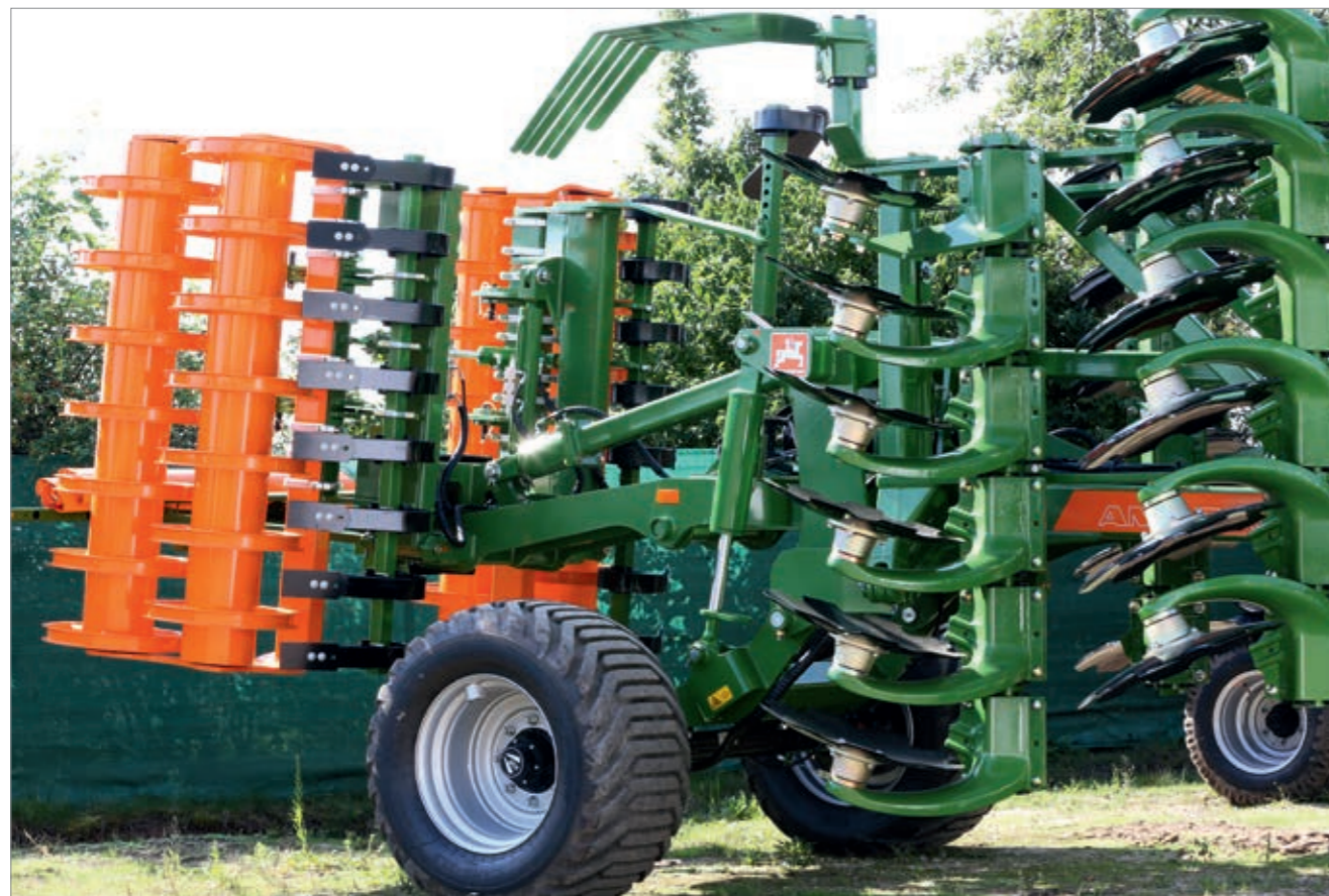
Images: © SELL MEDIA COMPANY - Norbert Sell - Catros 4001-2TX with double U profile roller
