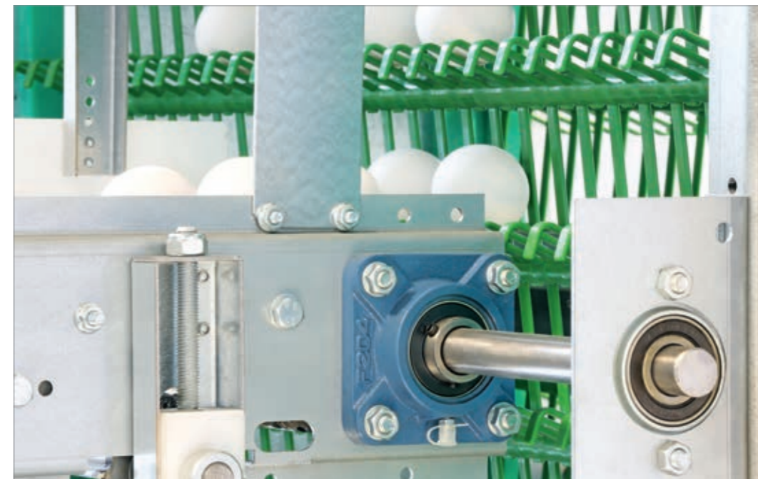
Guide unit for the crosswise egg collection
