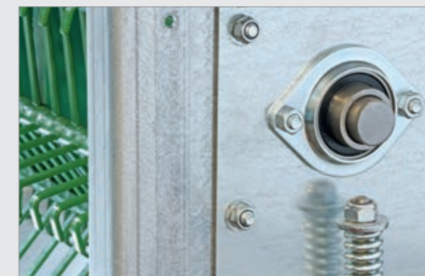
Flange bearing in a sheet steel housing in an egg elevator
